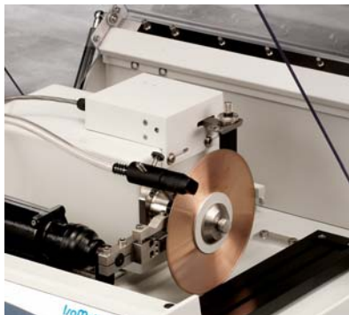
Samples can be positioned with 2µm accuracy with the IsoMet 5000's 11-2750 Precision 2µm Sample Positioning System. The 11-2683 stainless steel single saddle chuck, 11-2690 flange, and 11-2496 Chuck Padding shown.
