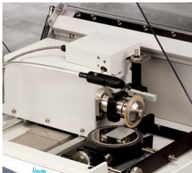
The 11-2694-115 Precision Table for sectioning thin materials rotates 180° in 1° increments to facilitate sectioning along a line of features on a die.
